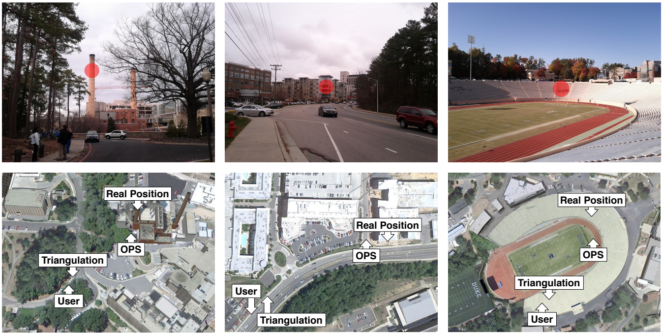
Figure 10: Sampled tests; circle denotes object-of-interest (top), Google Earth view (bottom): (a) smokestack of a coal power plant; (b) distant building with vehicles in foreground; (c) stadium seats near goal post.
